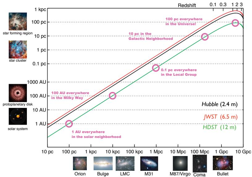
**Figure 2:** The physical size of *HDST*'s diffraction-limited spatial resolution element, as a function of distance/redshift. Note that the *HDST* resolution element is <100 AU anywhere in the Milky Way and <100 pc anywhere in the observable universe.
