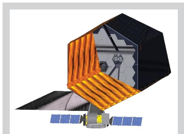
**Figure 1:** This is an artist’s concept of *HDST*, which will be a flagship 12-meter general observatory that combines exoplanet and cosmic origins science. It will feature broadband sensitivity, high-performance optical/NIR coronagraphy, far-UV multi-object spectroscopy, and unprecedented stability in support of high-precision astrometry, spectroscopy, and exoplanet characterization.
