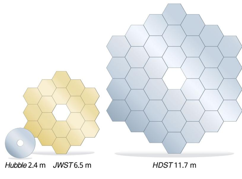
**Figure 3:** This is a direct, to-scale, comparison between the primary mirrors of *Hubble*, *JWST*, and *HDST*. In this concept, the *HDST* primary is composed of 36 1.7-meter segments. Smaller segments could also be used. An 11-meter class aperture could be made from 54 1.3-meter segments.
