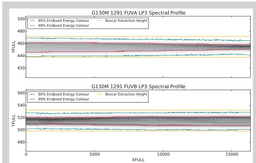
**Figure 4:** The point-source template reference profiles for both the FUVA (*top*) and FUVB (*bottom*) segments of the G130M 1291 setting at LP3 are shown by the grayscale images. Three sets of contours are also shown. The outermost yellow contours approximate the extraction region used in the BOXCAR algorithm. The blue curves mark the 99% enclosed energy contour, while the red curves show the 80% enclosed energy contour.
