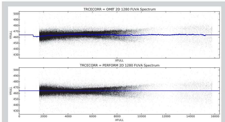
**Figure 2:** This figure shows how the new distortion correction in the revised algorithm removes optical and detector distortions, yielding a straighter spectrum that is easier to compare and align with reference profiles. The *top* panel shows the uncorrected spectral image for a G140L 1280 FUVA observation, while the *bottom* panel shows the image after the correction has been applied.
