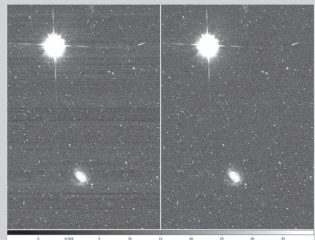
Figure 2: *Left*: A 2013 ACS sub-array image processed with the default CALACS pipeline. *Right*: The same image, processed with the ACS\_DESTRIPE\_PLUS script, which combines CTE correction and the stand-alone de-stripe code with object masking.
