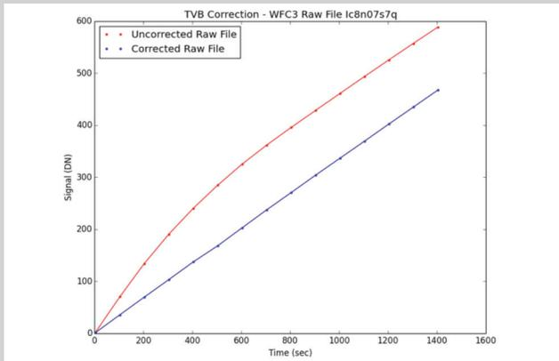
**Figure 3:** The red curve shows the original reads from image ic8n07s7q, while the blue curve shows ic8n07s7q after performing the TVB correction, returning the background to a linear function. Data courtesy of Harish Khandrika.
