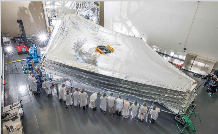
**Figure 1.** Picture of the full-scale sunshield model after the first successful unfolding test. This is an engineering version of the five-layered sunshield, pictured during tests at Northrop Grumman in July 2014. Manufacturing of the flight versions of individual layers is occurring in tandem. (Credit: NASA/Chris Gunn.)
