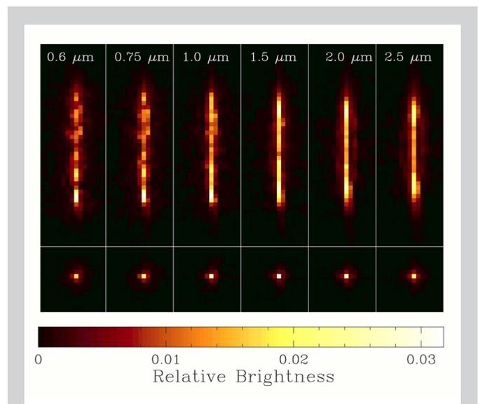
**Figure 2:** Simulation of the SOSS cdPSF (the PSF in the direction perpendicular to the dispersion). The top panels depict simulations at the wavelengths indicated with the weak lens in place, while the bottom panels do so *without* the weak lens. The features shown in these simulations have been confirmed by actual observations taken during the cryogenic vacuum tests at Goddard Space Flight Center. (Figure courtesy of David Lafrenière, Université de Montréal).
