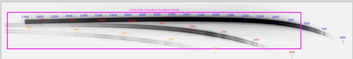
**Figure 1:** Simulation of the appearance of a SOSS spectrum of a M3V star. Grayscales indicate intensities in logarithmic units. Wavelengths in nm are indicated in blue, red, and orange for spectral orders 1, 2, and 3, respectively. The magenta box outlines the portion of the spectrum read out by the default SOSS detector window.
