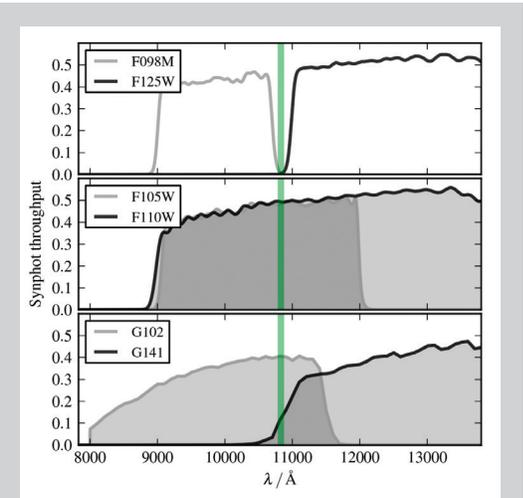
Figure 3: The F105W and F110W filters and both infrared grisms are sensitive to the He line at 1.083 microns. The F098M and F125W filters are not.
